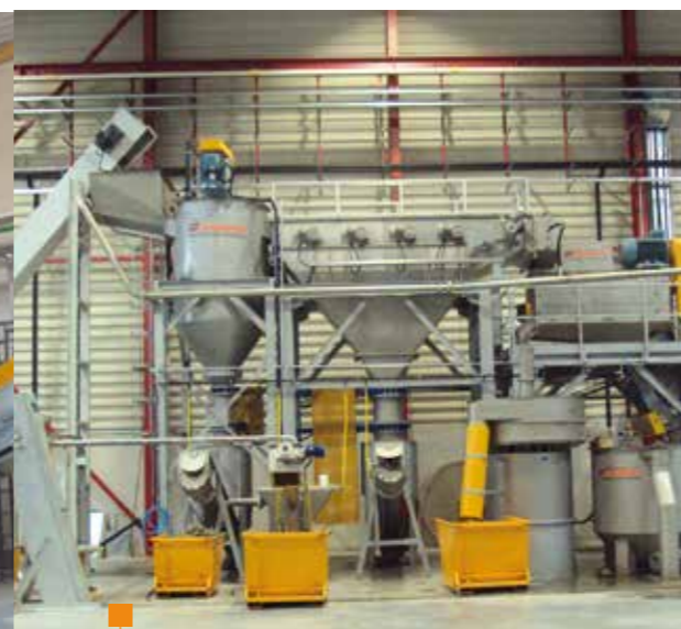
FILM PREWASH: DIFFERENT SOLUTIONS ACCORDING TO CONTAMINATION. BY REDUCING MAJORITY OF CONTAMINANTS INCREASE PERFORMANCE OF WASH LINE.
