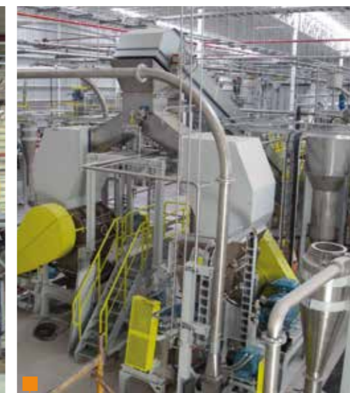
WET GRINDER: UNITS WITH HIGH FLEXIBILITY AND PERFORMANCES FOR EVERY TYPE OF PLASTICS. SPECIAL DESIGN WITH INTERCHANGEABLE WEARING PARTS.
