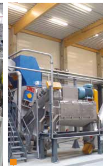
WET GRINDER: UNITS WITH HIGH FLEXIBILITY AND PERFORMANCES FOR EVERY TYPE OF PLASTICS. SPECIAL DESIGN WITH INTERCHANGEABLE WEARING PARTS.
